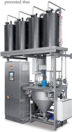
maximizing reproducibility. Down time also is avoided because the systems can prepare the dyes, chemicals and auxiliaries in advance. The synchronized system and production sequence ensures each product is available in the right quantity at the right time at the right machine.
